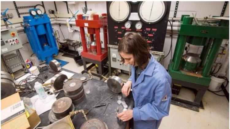
In her laboratory experiments, Sarafian used a piston-cylinder apparatus--the red machine behind her--to simulate the high pressures and temperature of the Earth's mantle. The heavy stainless steel plates visible on the table are stacked on the apparatus, with the tiny synthetic mantle sample inside a 'pressure vessel' underneath them. Once the machine is turned on, pistons apply massive pressure from above and below the sample, which is simultaneously heated with electrical current.
