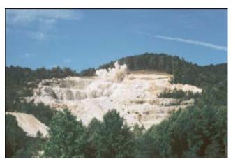
The photo to the left was taken recently when a shelf of pegmatite was being blasted at the Wakefield Mine in Spruce Pine, NC.
